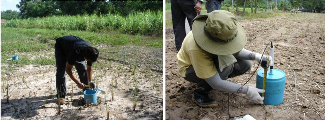
**Figure 4** Soil chamber (left) and measurement of CO<sub>2</sub> emission rate by using a Hand-Held CO<sub>2</sub> Meter (right)
