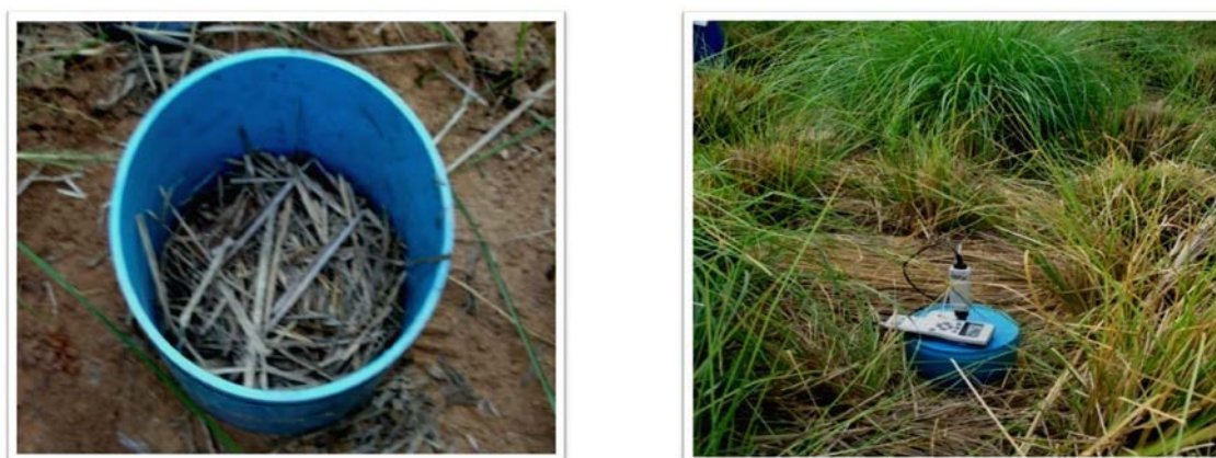
Figure 4 Gas chamber (left) and measurement of CO 2 emission rate by Hand-Held CO 2 Meter (right)
